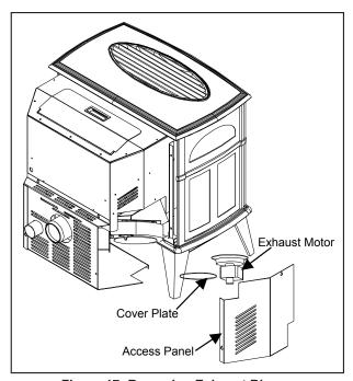
Figure 17: Removing Exhaust Blower.
